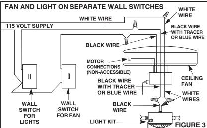
If combined weight of light kit and ceiling fan exceeds 35 pounds, fan should be supported independently from the outlet box. Check the following list for the weight of the light kit.
